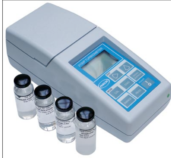
Figure 5-1: Hach 2100P turbidimeter (Filtration Technology Ltd.)
