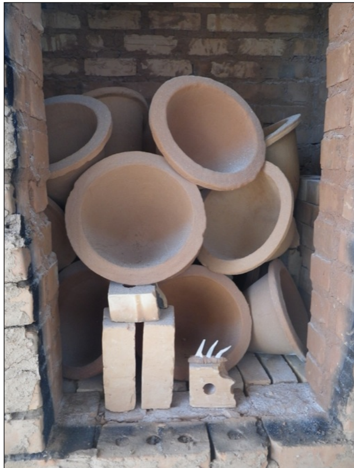
Figure 4-15: Filters stacked in kiln (Manny Hernandez)
