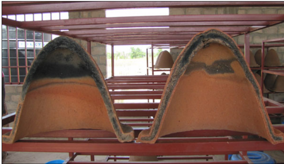
Figure 7-4: Incomplete firing (cross section)
