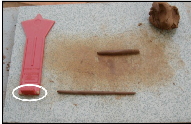
Figure 3-18: Bottom of grooving tool (circled) used as guide for rolling to 1/8 in.
