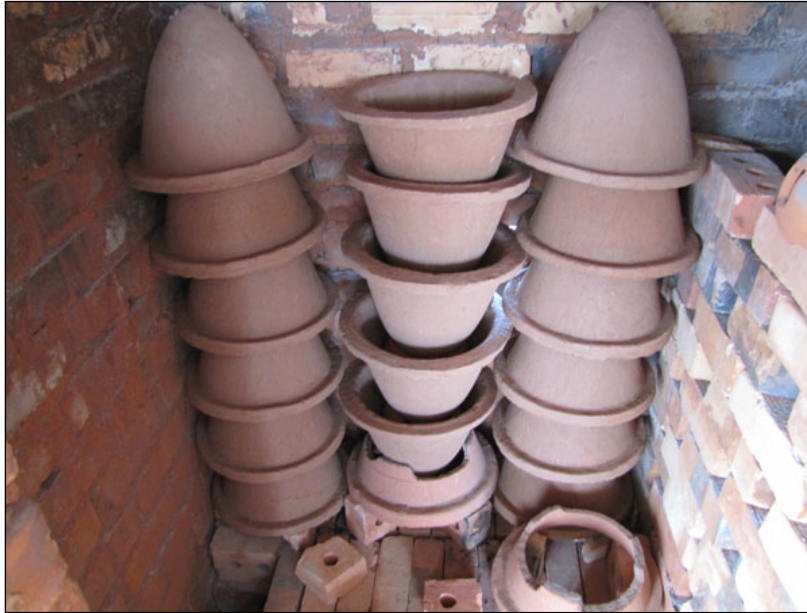
Figure 7-1: Filters stacked in kiln with first revised spacer
