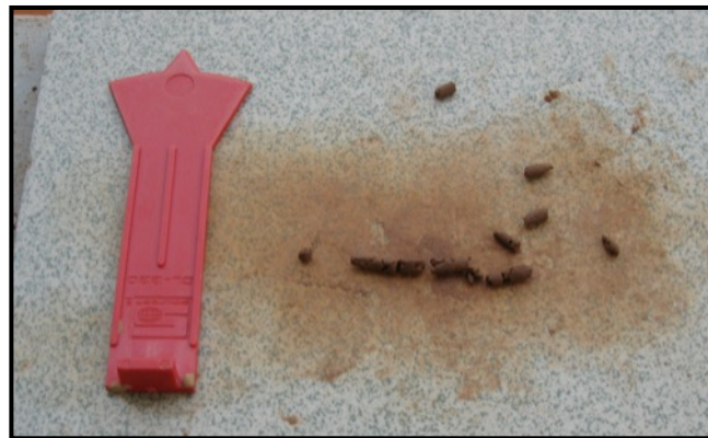
Figure 3-19: Clay thread crumbling at 1/8 in.
