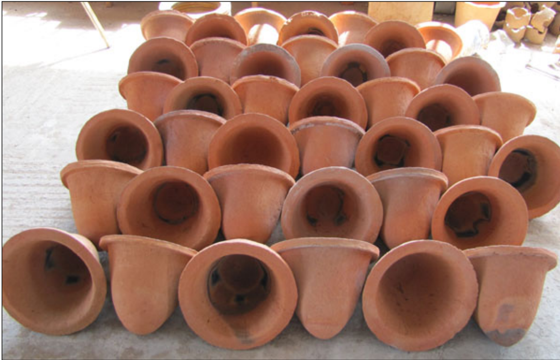
Figure 7-3: Incomplete firing using first spacer revision
