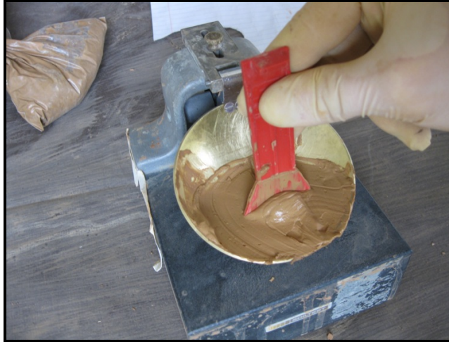
Figure 3-13: Grooving the pat of soil
