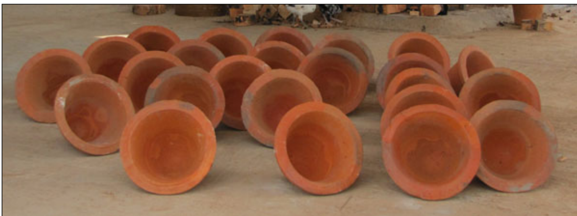
Figure 7-6: Completely fired filters after using new spacers
